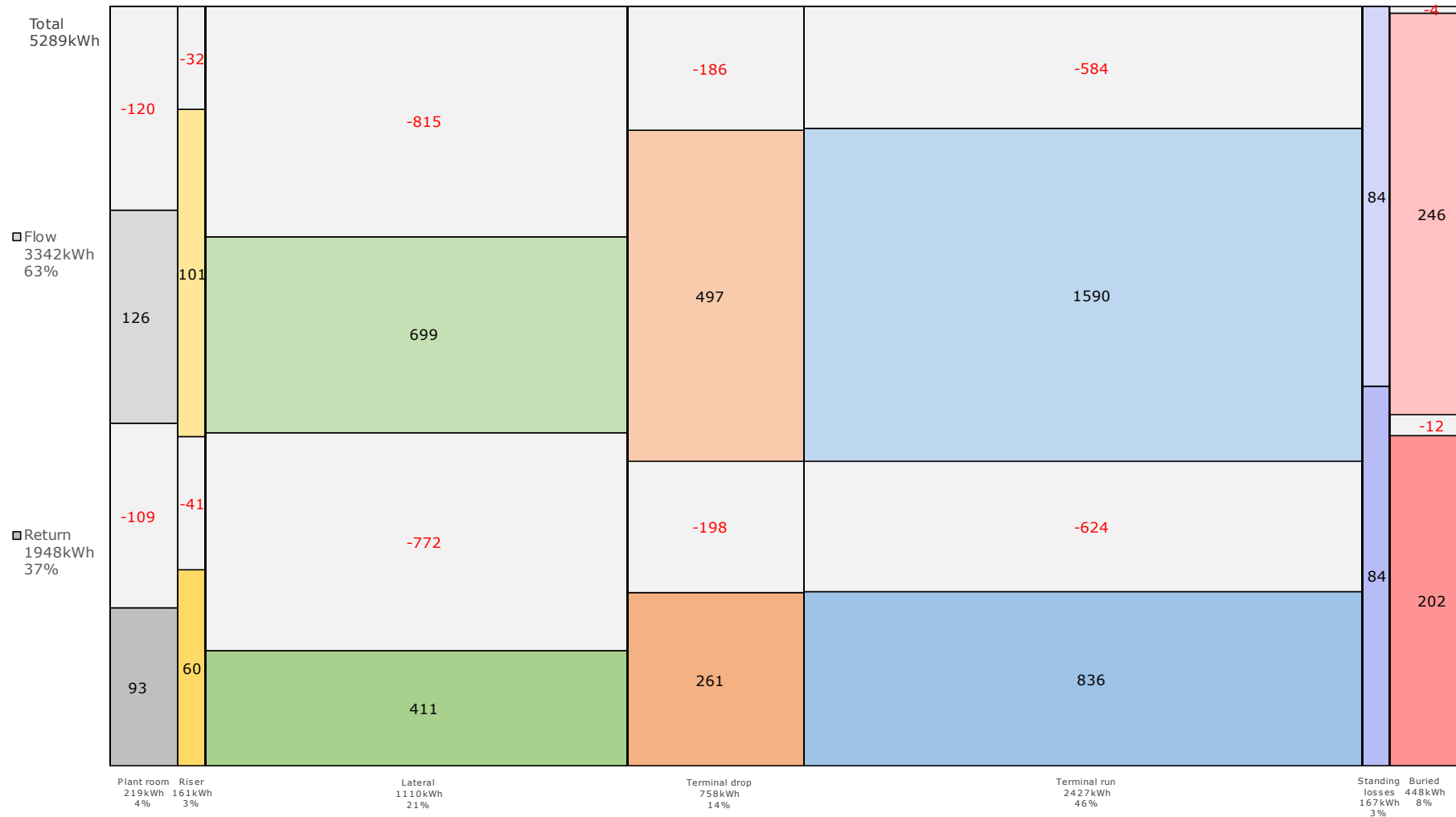
Figure 7: The results of a heat loss model detailing the Work Package 1 kWh heat losses per resident per annum broken down into pipework sections and flow and return pipework
